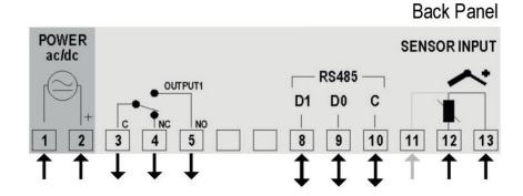
Pt1000 with 3 conductors: Terminals 11, 12 and 13 must have the same wire resistance for proper cable length compensation. For 2 wire Pt1000, short circuit terminals 11 and 12.
